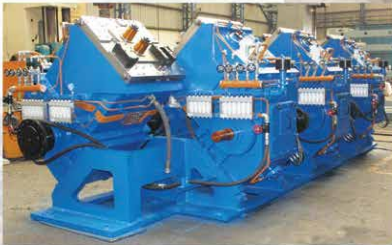
Block Mill supplied to Shree Steel, Nepal for Ø8-Ø20mm TMT rebars
