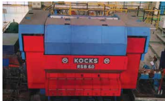
The RSB® 370++/4 is located as a finishing unit after 20 stands in H/V rolling mill arrangement
