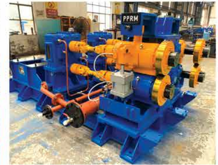
Tail Breaking Pinch Roll @ 40mps
