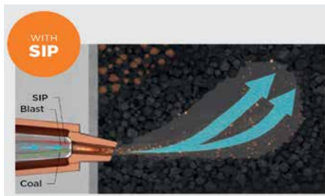
Fig. 3: With SIP implemented, the shock waves from the high-pressure oxygen penetrate deep into the raceway, combusting the fine char and improving coke permeability
