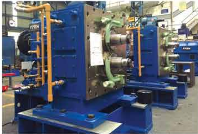
Cantilever Stands for TMT Bar from TC Rings with groove life of 800 – 1000 Tons @ 24mps
