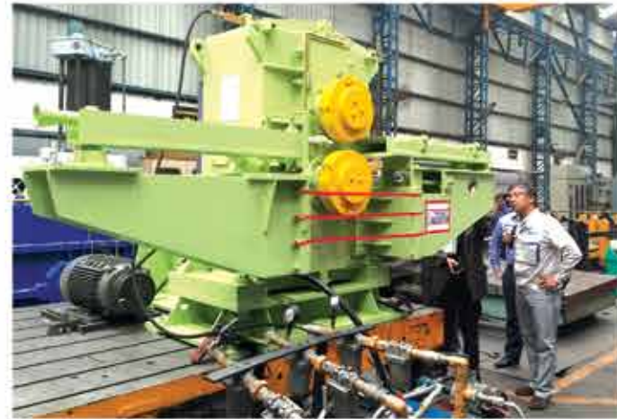
Continuous Operating Shear to cut 8mm rebar to 16mm in High Speed exported to KOBELCO Japan
