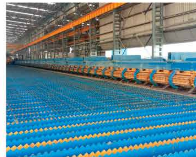
High Speed Rotating Drums can handle 8mm Rebars @ 40mps
