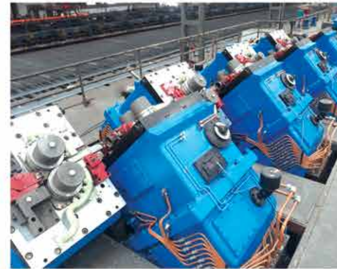
100 mps Wire Rod Block Designed by KOBELCO Japan successfully Commissioned at JAIDEEP, INDORE
