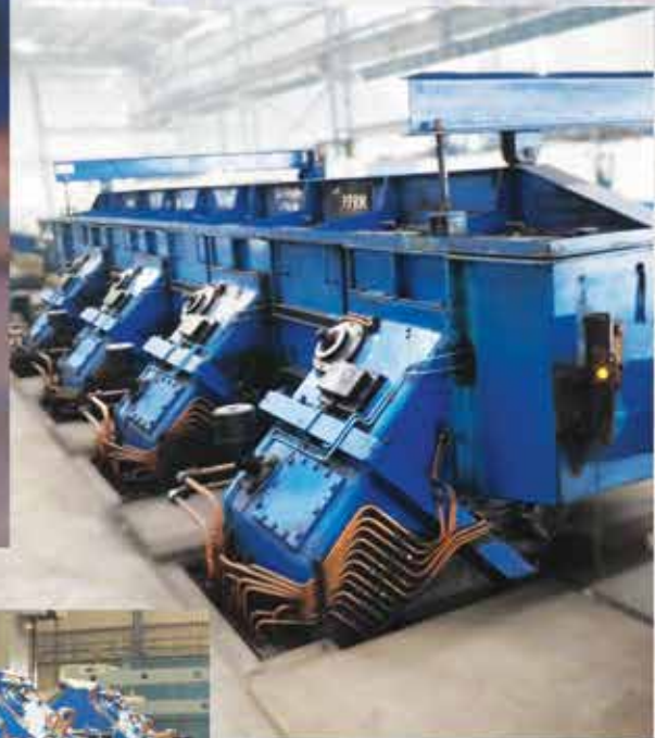
Block Mill supplied to Madhav Steel Punjab, India for Ø5.5mm Wire Rod @85mps
