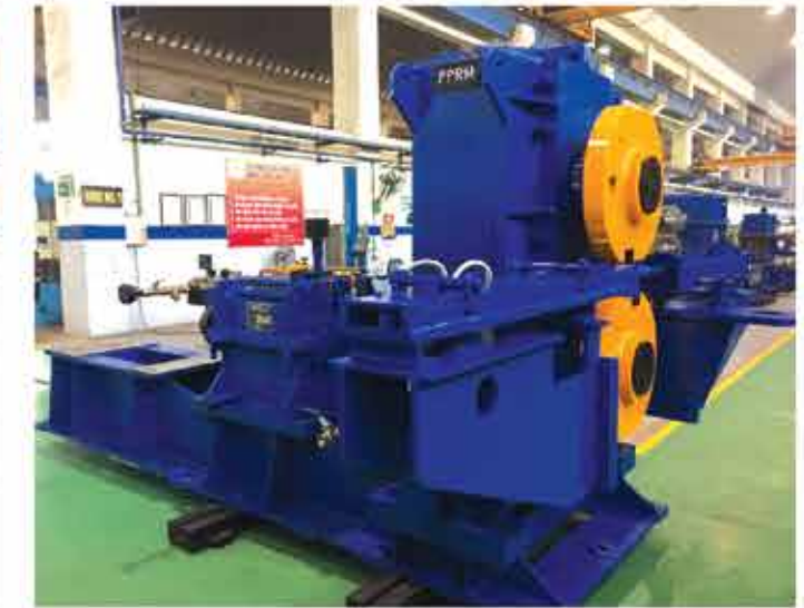
Combination Shear to cut 8mm to 40mm with 8mm @ 40mps and 40mm @ 2mps
